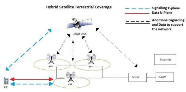
Fig. 1. Hybrid satellite terrestial system architecture
