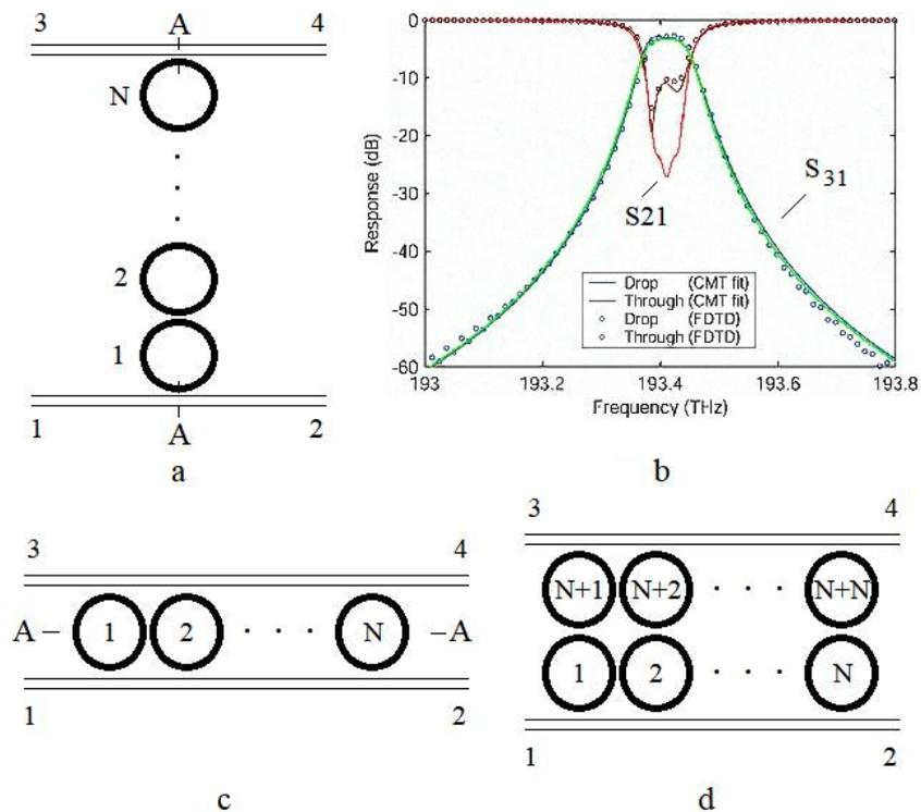
Fig. 1. Different add-drop filters (a, c, d) on microresonators. Comparison of S-matrix of the 3-microresonator filter from [4]; calculated by theory [9]:  $S_{21}$  - red;  $S_{31}$  - green curve
