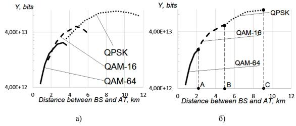
Fig. 2. Productivity *Y* for coverage area with QAM MPK types,  $p_b=10^{-6}$ ,  $n_{LDPC}=1000$  (a) and maximal coverage productivity and points of MPK types / antinoise code switching (b)
