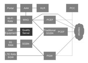
Fig. 1 Wi-Fi offload arcitecture scheme
