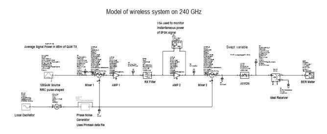
Fig. 1 The model wireless system
