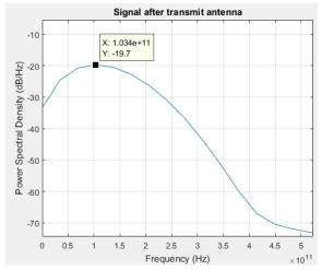
Fig.2. Spectral density of pulse in channel.
