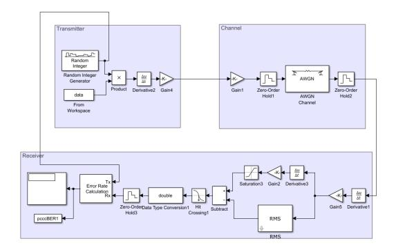
Fig.3. Functional diagram of IR-UWB system.
