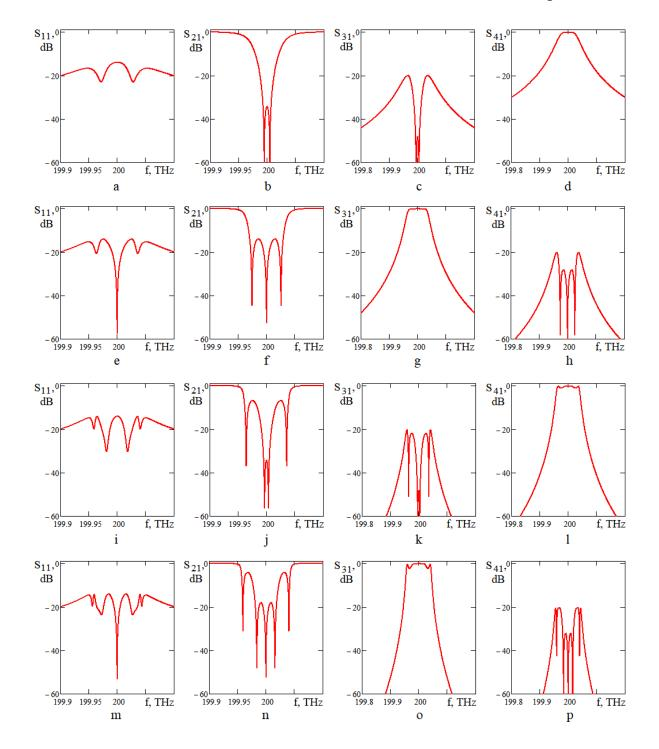
Fig. 2. Example of calculated dependences of scattering matrices of the Add-Drop Filters, shown in fig. 1, a, on 2 (a - d); 3 (e - h); 4 (i - l); 5 (m - p) microresonators.
