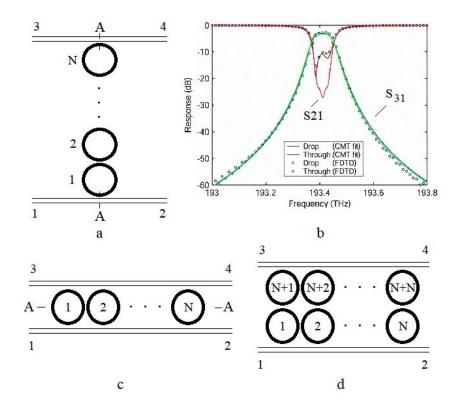
Fig. 1. Different add-drop filters (a, c, d) on microresonators. Comparison of S-matrix of the 3-microresonator filter from [4]; calculated by theory [9]:  $S_{21}$  - red;  $S_{31}$  - green curve
