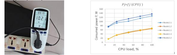
Fig. 3. Preliminary cluster evaluation: 1 – wattmeter for  $P_j = f_j(CPU_j)$  defining; 2 -  $P_i = f_i(CPU_j)$  functions got experimentally.
